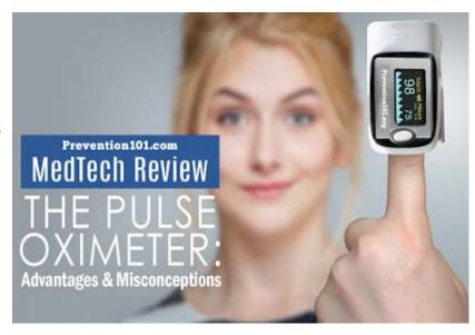
THE PULSE OXIMETER- is an electronic device that clips onto a patient's finger to measure heart rate and oxygen saturation in his or her red blood cells—the device is useful in assessing patients with lung disease.
